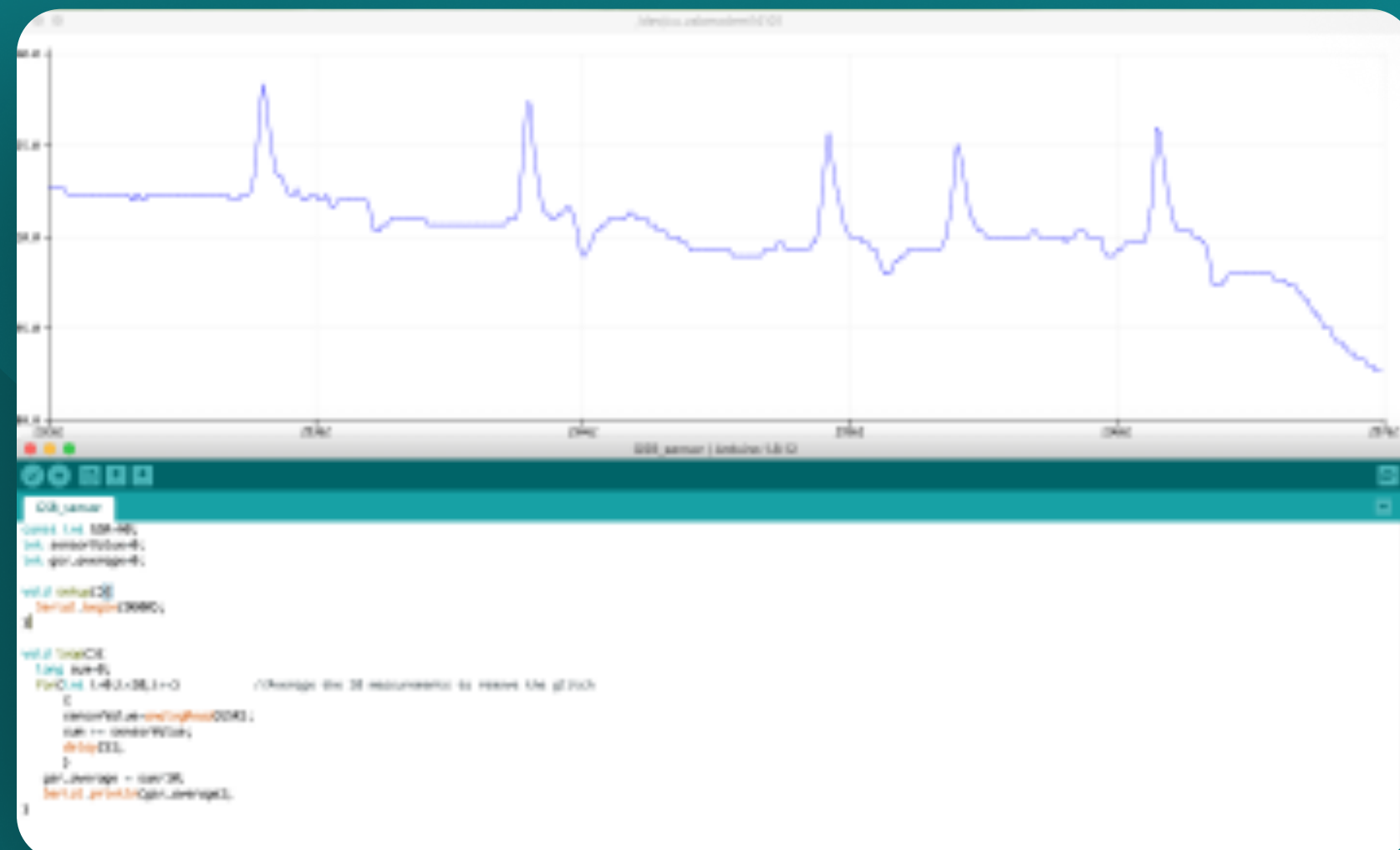
2 The figure varied greatly when the user keeps standing up and sitting down
